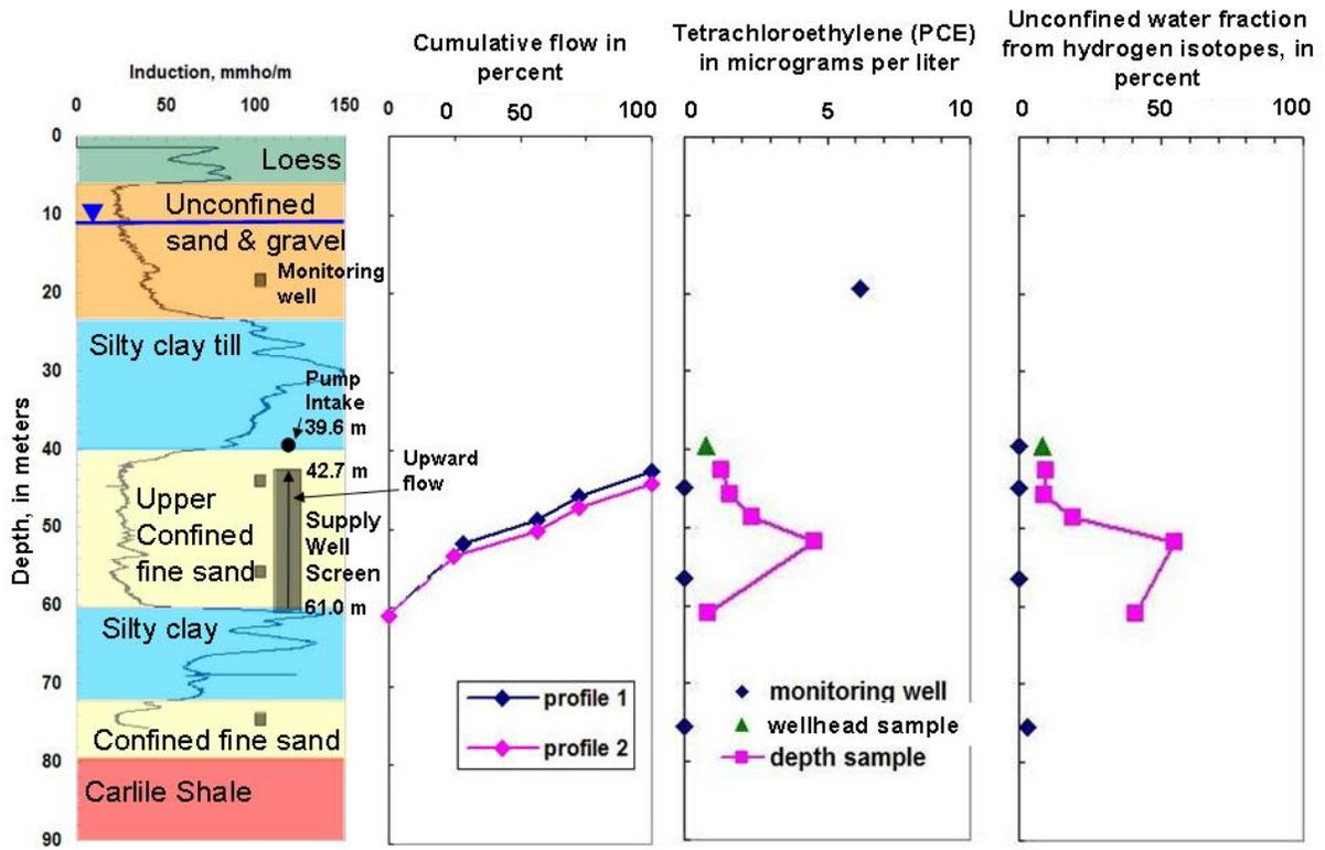
Figure 4. High Plains aquifer study-area depth-dependent results: lithology, induction log, and well construction, percent cumulative flow in public-supply well screened interval, PCE concentrations, and unconfined water fraction from mixing fractions with hydrogen isotopes.
