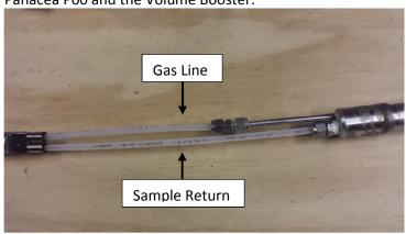
Photo showing Volume Booster connected to tubing.
